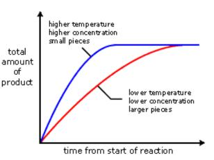
The reaction stops when one of the reactants (the limiting factor) gets used up and the graph goes flat.
